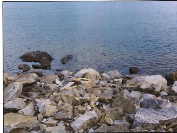
Photo 13. View of boulder and cobble substrate overlying bedrock in front of Lot 1.
