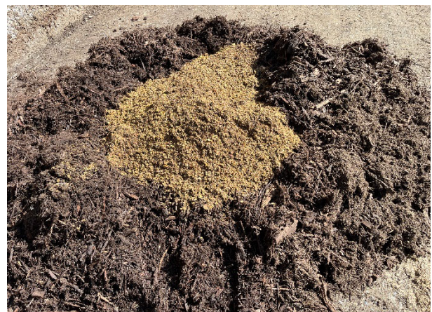
Figure 3. 25 kg of dried and ground food scraps with the 294 kg bulking agent.
