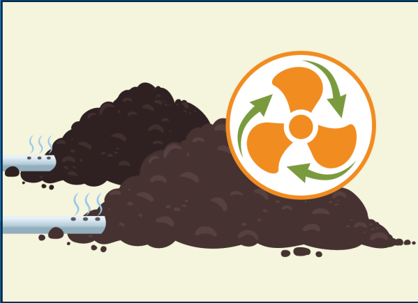
Aerated Compost Windrows— fans connected to aeration piping blow air into the windrows, which maintains ideal oxygen and temperature for decomposition.
