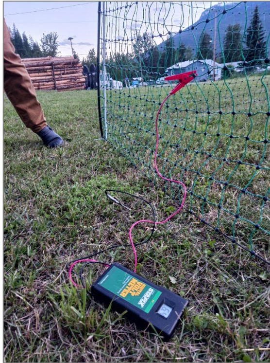
Figure 16. Testing the voltage of the demonstration electric fence at the New Denver electric fence workshop.
