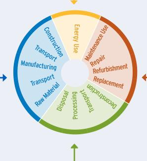
**Embodied Carbon Emissions** is carbon pollution associated with materials and construction processes throughout the whole lifecycle of a building. As shown above, this can be a significant percentage of the building's total carbon pollution.
