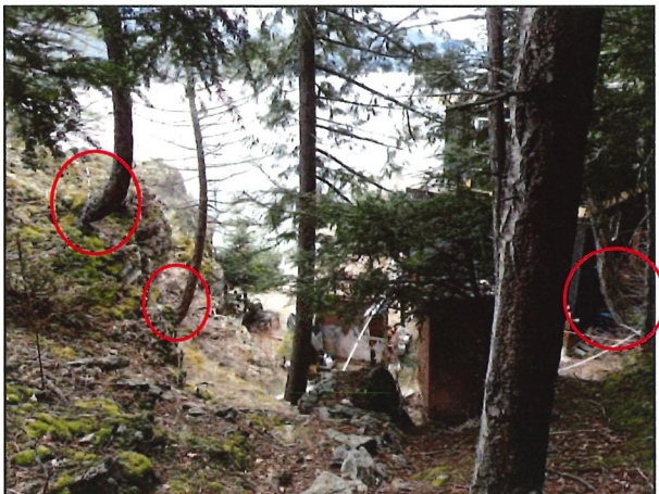
Photo 16. Slope mobility over a longer time period evidenced by sweeping/curved tree trunks growing on the slopes to the north and west of the cabin
