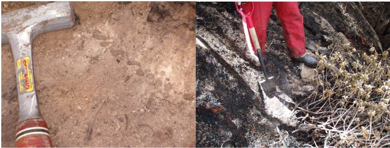
Photos 4 and 5 Water drops sitting on soil trench (left) dug to test for water-repellency, demonstrating non-infiltrating water. Right - water trapped above water repellent layer after small recent rainfall in Allen Creek – Allen Creek Watershed
