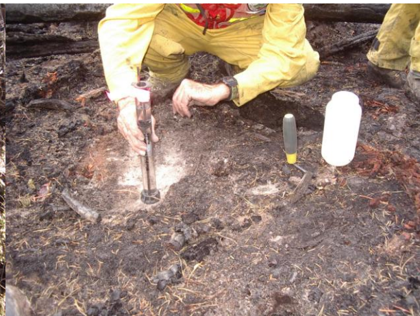
Photo 10 Infiltrometer Test – Cory Creek Watershed
