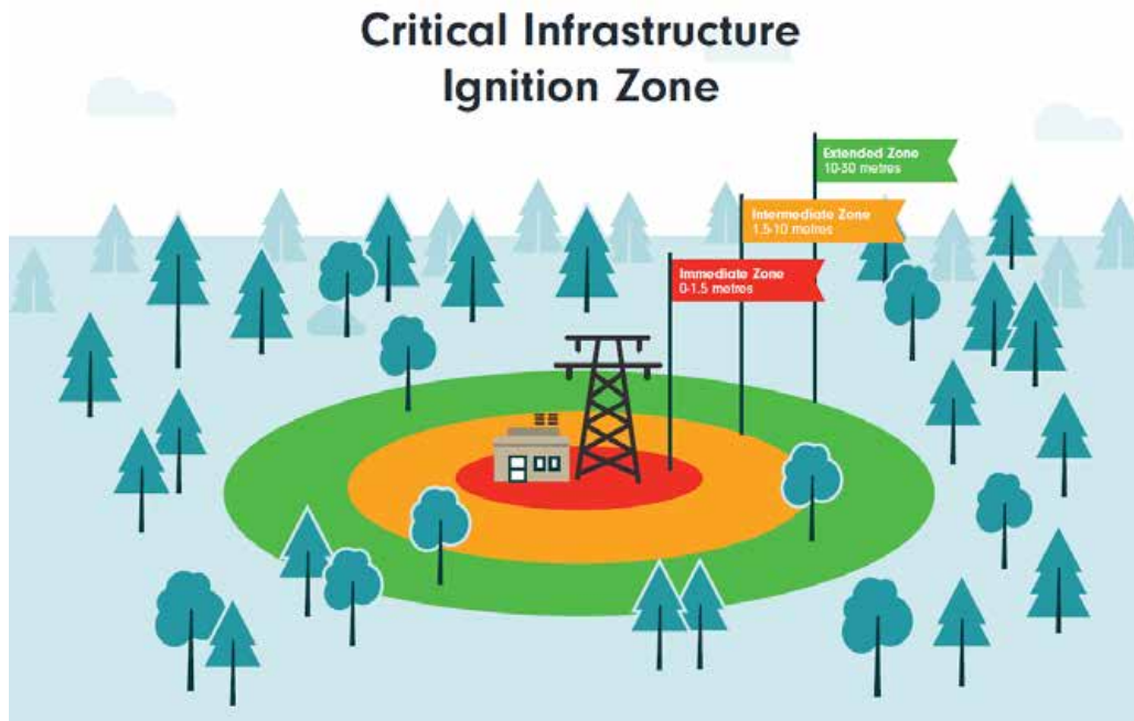
Figure 15: FireSmart Home and Critical Infrastructure Ignition Zone (HIZ, CIIZ)
