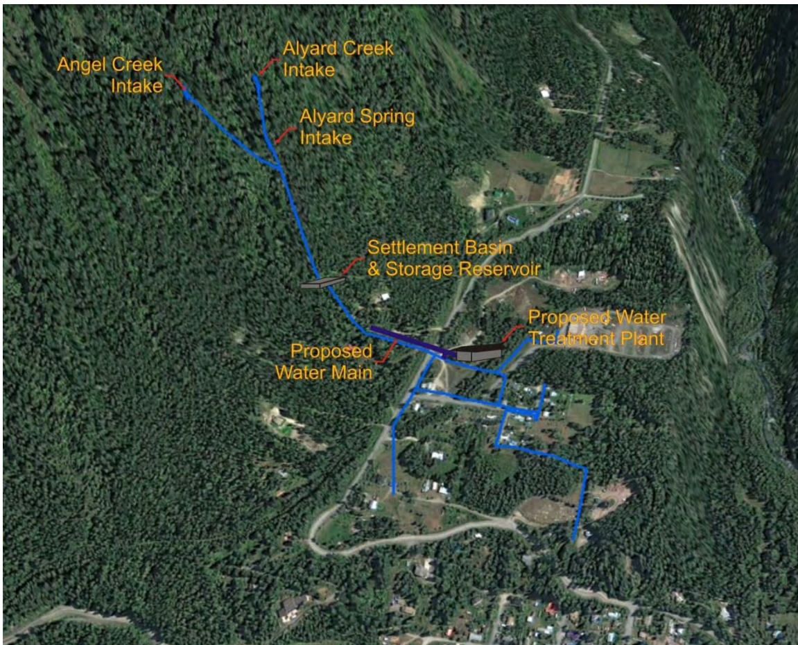
Figure 5: Central Treatment Plant Downstream of Reservoir
