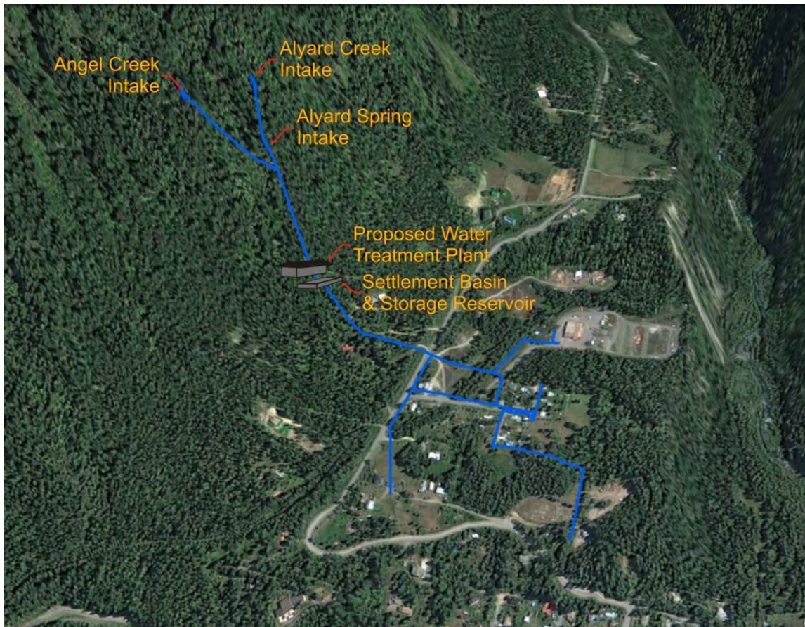
Figure 5: Central Treatment Plant Adjacent to Reservoir
