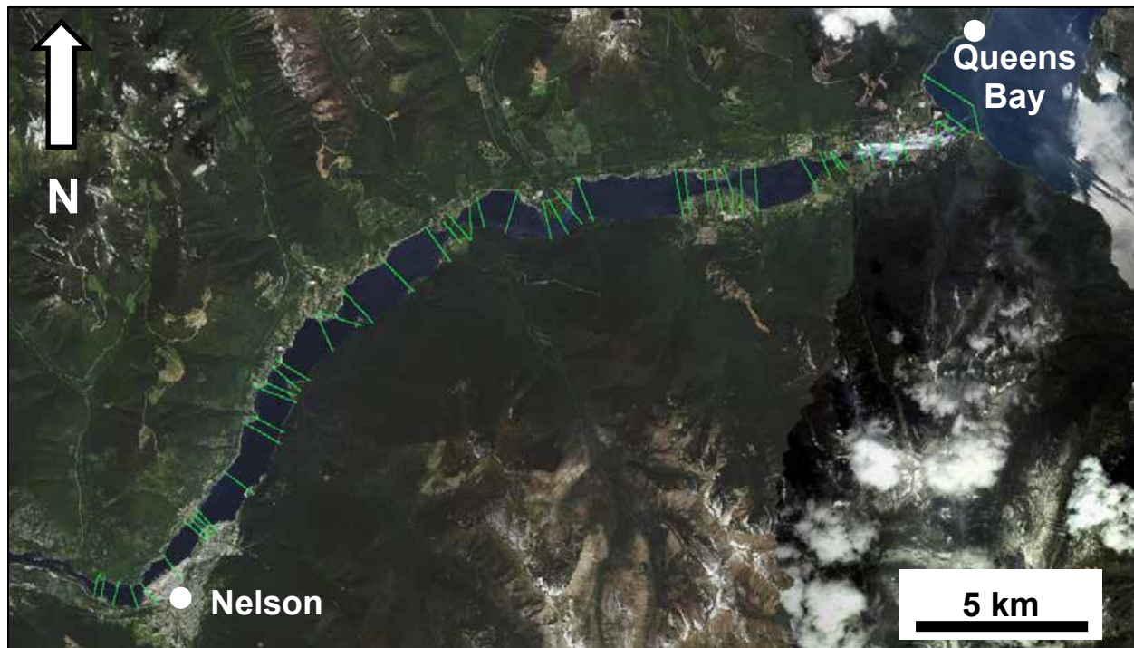
Figure 3-1. Cross sections (green) used for 1-dimensional hydraulic modelling along the West Arm.
