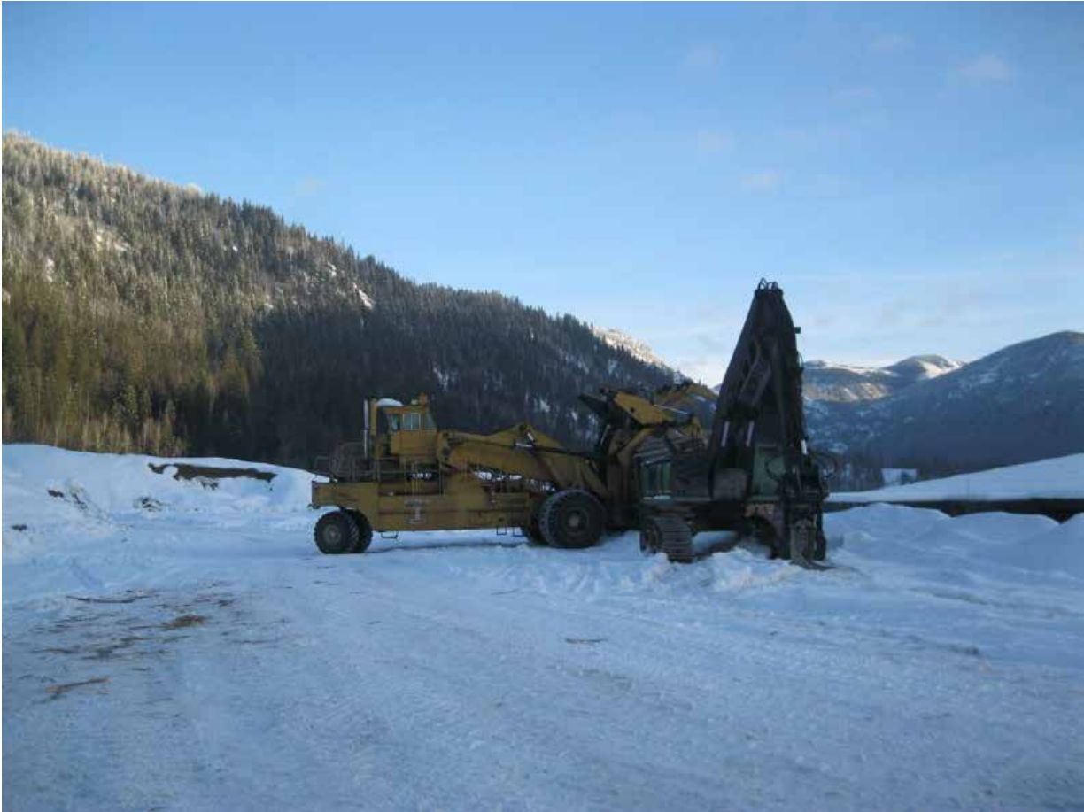
Figure 4: 'The Wardner' (left-most machine)- This machine cannot operate on a slope
