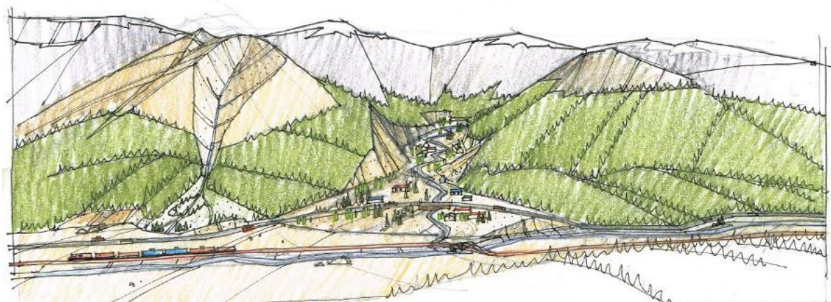
Figure 1-3. Typical steep and low-gradient fans feeding into a broader floodplain. On the left a small watershed prone to debris flows has created a steep fan that may also be subject to rock fall processes. On the right a larger watershed prone to debris floods has created a lower gradient fan. Development and infrastructure are shown to illustrate their interaction with steep creek geohazard events. Artwork: Derrill Shuttleworth.
