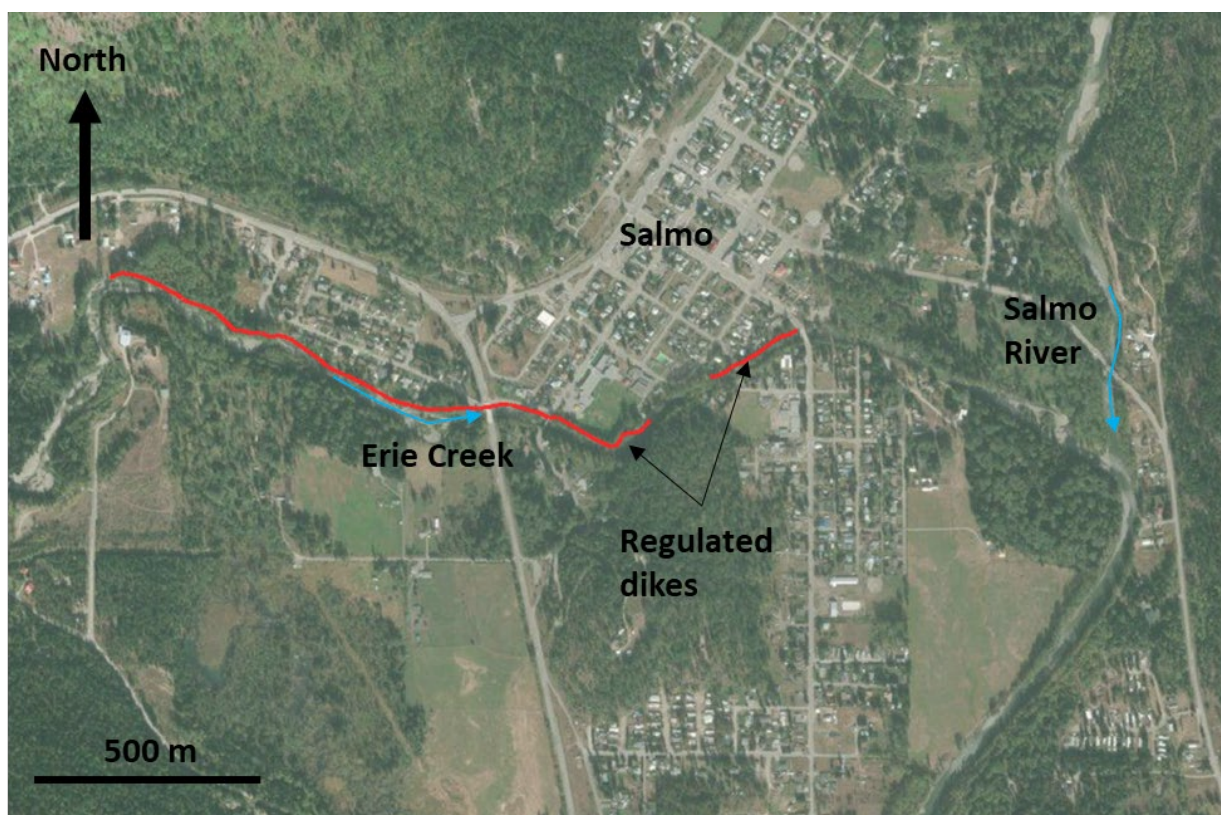
Figure E-20. Regulated dikes along the left (north) bank of Erie Creek. Satellite imagery from Bing.
