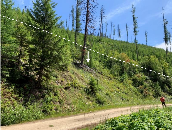
Photo 8. Looking east on Redfish-Liard Creek FSR at overgrown side scarp (dashed line) of debris avalanche. Note arrow pointing to rounded granitic boulders contained in till. See Drawing 05 for location. Photo: BGC, July 10, 2019.
