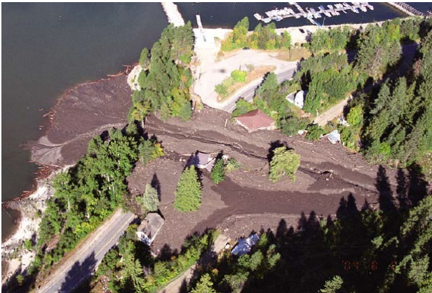
C) August 2004 debris flow deposit on Kuskonook Creek fan-delta. P. Jordan photo.
