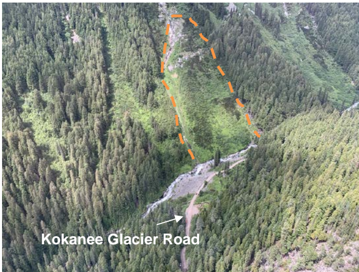
Photo 5. Overview photo taken during helicopter overflight looking down (west at the top) at the lower Kokanee Creek watershed, approximately 8 km upstream of the fan apex. Kokanee Glacier Road is visible, as well as the site of a potential debris avalanche (orange) to the west of the creek. Photo: BGC, July 6, 2019.
