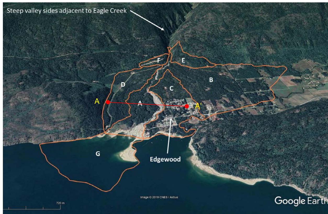
Figure 3-4. Oblique view of the Eagle Creek fan-delta looking west. Edgewood is located on the mid to distal end of the fan-delta. Areas A through G refer to geomorphic surfaces described in text. Photo: Google Earth (2019). The cross-section A-A' related to Figure 3-3.
