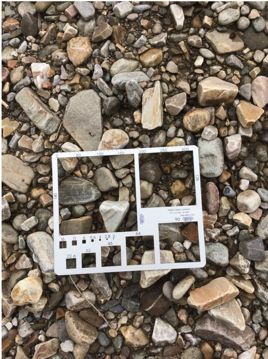
Photo 14. Woolman sample of Bed Material immediately north of the Highway 3A bridge. Photo: BGC, July 4, 2019.
