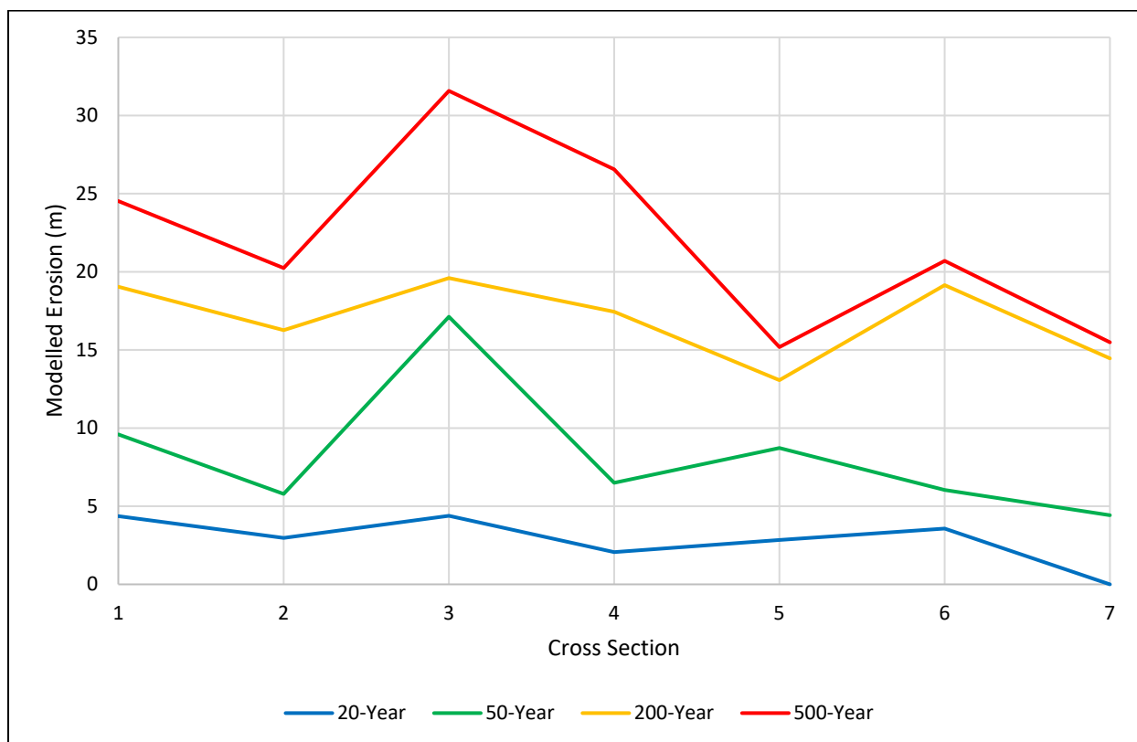
Figure 6-2. Cooper Creek 50 th percentile bank erosion model results at each cross-section.
